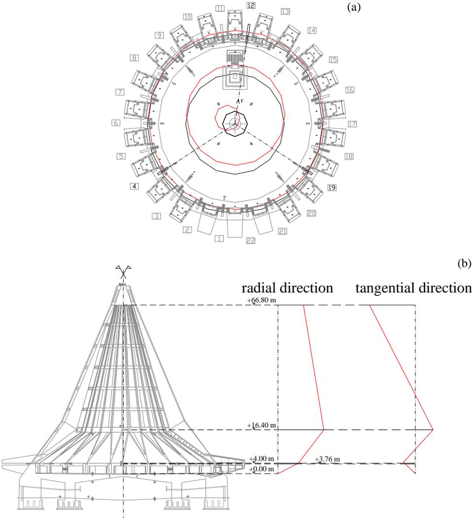
**Figure 2.4.** Mode shape at 3.78÷3.85 Hz: plane view (a), vertical section by column ⑫ (b)
