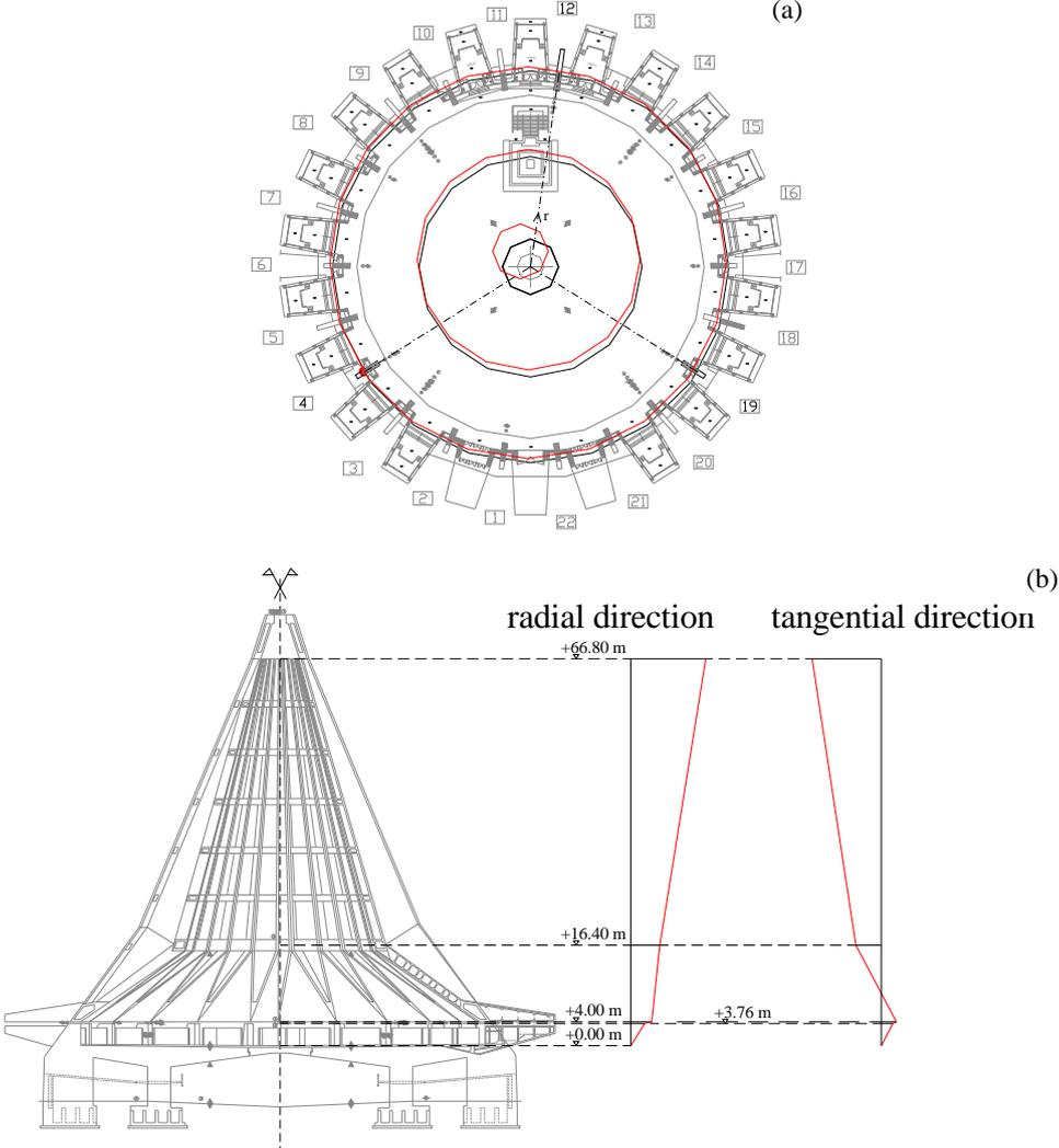
**Figure 2.3.** Mode shape at 2.88÷2.98 Hz: plane view (a), vertical section by column ⑫ (b)
