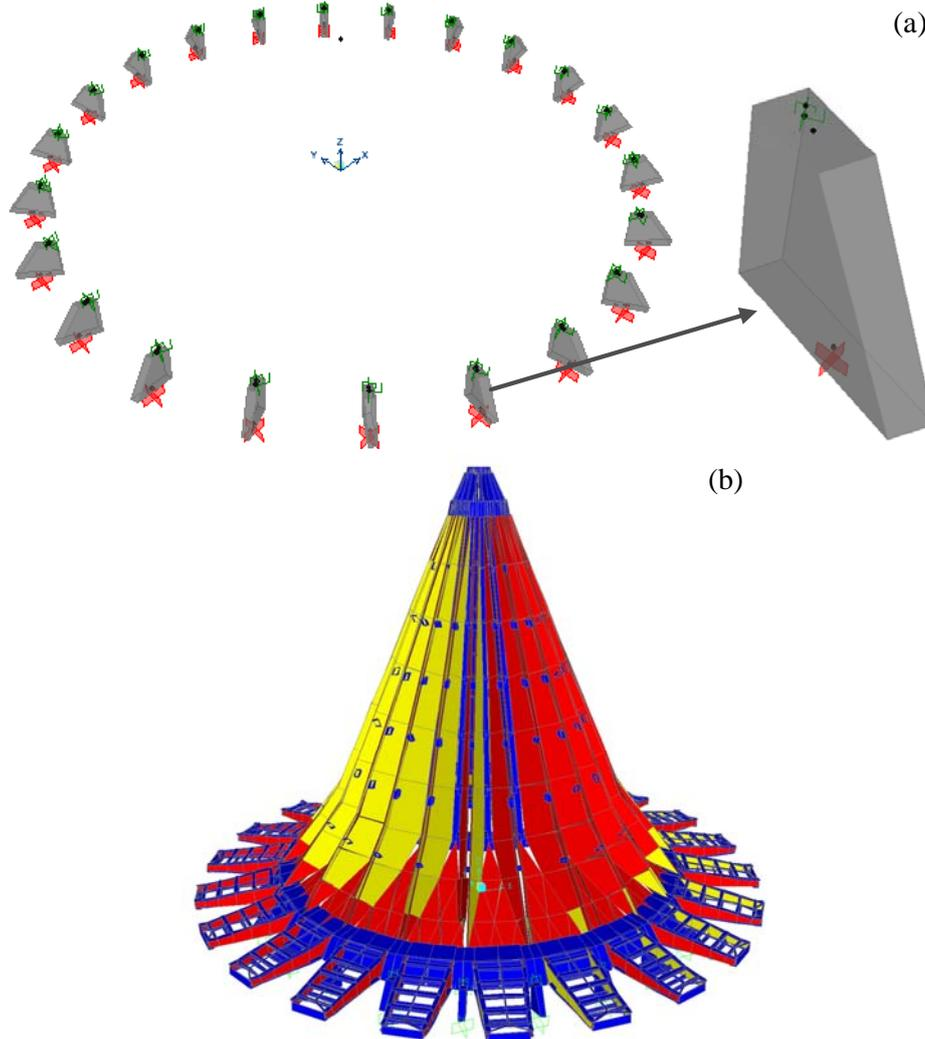
**Figure 1.5.** Simplified numerical model (a), complete numerical model (b)
