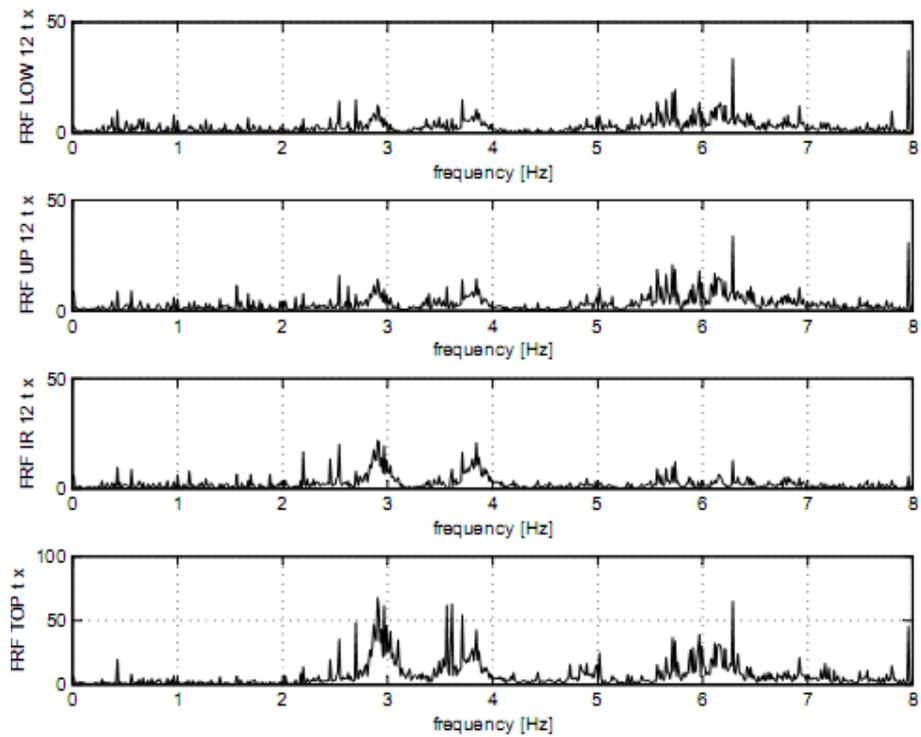
**Figure 2.2.** FRFs computed at column ② respect to input along x
