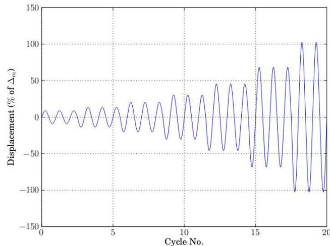
**Figure 2.2.** Time history of applied load on test structures
