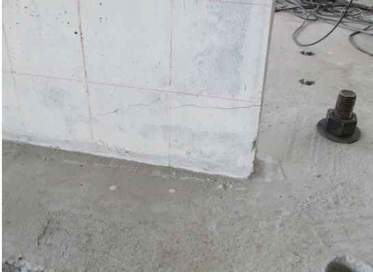
(b) Fracture at the edge of module (0.20% drift)
