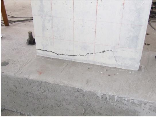
(e) Fracture at the base (0.85% drift ratio)
