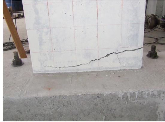
(f) Fracture at the base (1.00% drift ratio)
