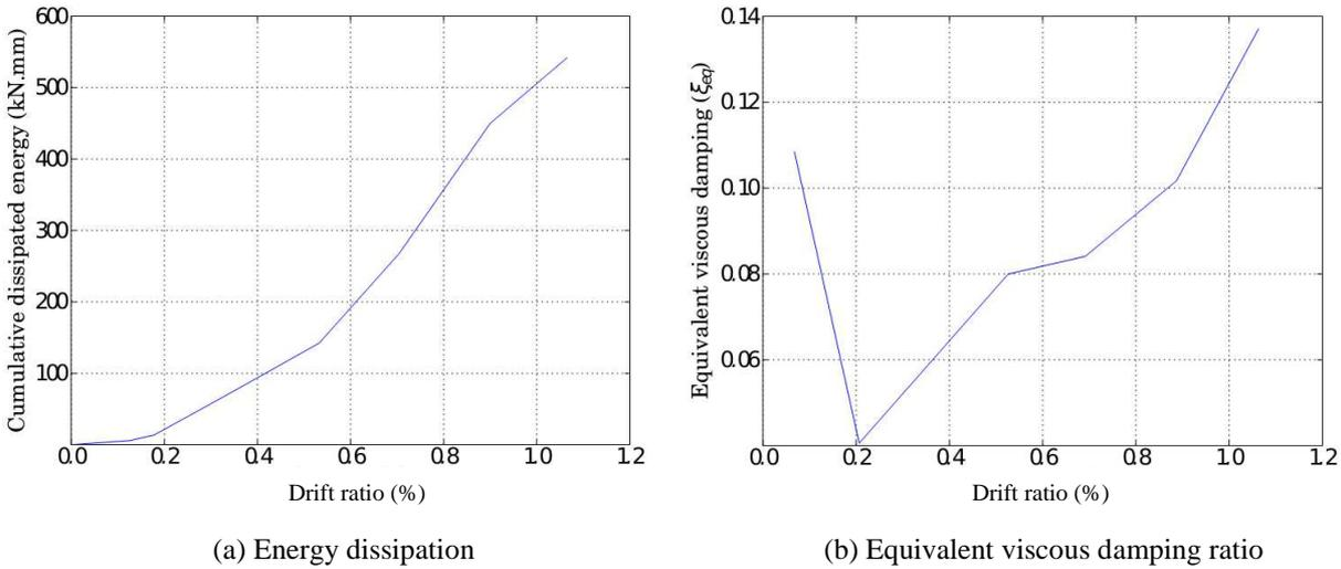
**Figure 3.3.** Energy dissipation and damping
