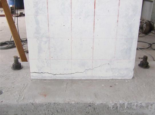
(c) Fracture at the base (0.55% drift ratio)
