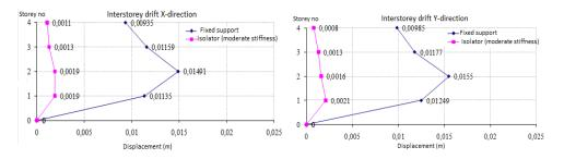
Figure 3.9 Interstorey displacements in both X and Y directions for both the original and the base isolated structures
