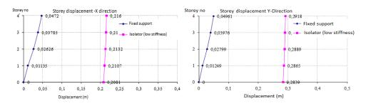
Figure 3.1 Storey displacements in both X and Y directions for both the original and the base isolated structures
