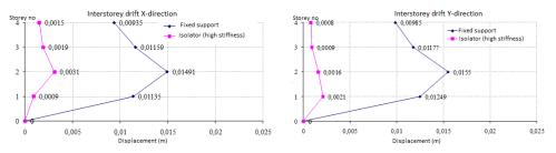
Figure 3.16 Interstorey displacements in both X and Y directions for both the original and the base isolated structures
