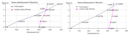
Figure 3.15 Storey displacements in both X and Y directions for both the original and the base isolated structures
