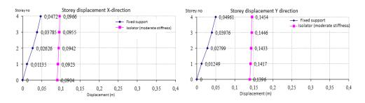
Figure 3.8 Storey displacements in both X and Y directions for both the original and the base isolated structures
