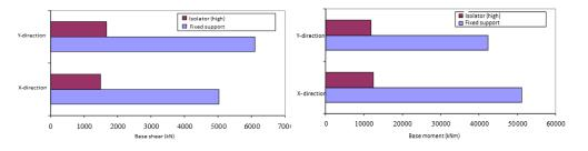
**Figure 3.21** Base shear forces and base flexural moments for both the original structure and the base isolated structure
