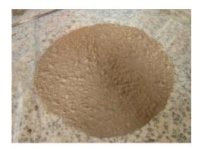
Figure 2.6. The Slump test
