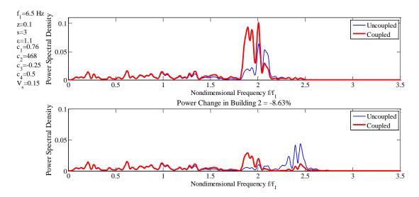
Figure 4.2. Response power spectra for total sway displacements for buildings 1 and 2 due to Westmorland earthquake.
