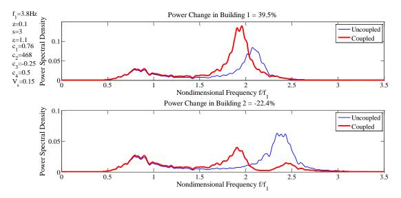
Figure 4.1. Response power spectra for total sway displacements for buildings 1 and 2, due to Kanai-Tajimi excitation.
