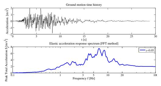
**Figure 3.2**. Ground motion time history (horizontal component) and its elastic acceleration response spectrum – Westmorland earthquake, PGA=1.95 [m/s<sup>2</sup>].
