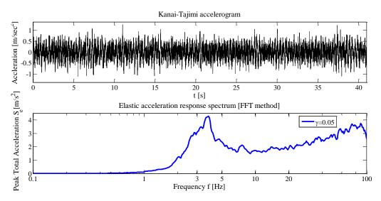
Figure 3.1. Kanai Tajimi artificial accelerogram and elastic acceleration response spectrum (5% damping).
