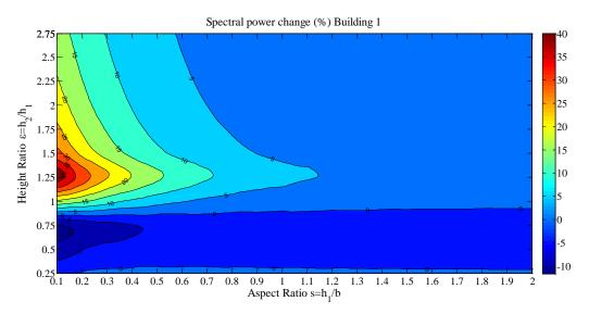
**Figure 4.5.** Change in power (caused by coupling) vs. height ratio  $\varepsilon$  and inter-building spacing *z*, *s*=3.25 - Kanai-Tajimi
