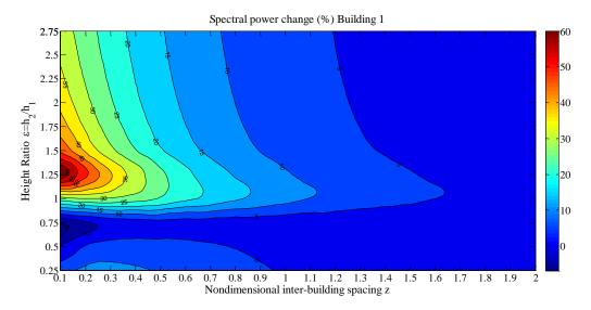
**Figure 4.6.** Change in power (caused by coupling) vs. height ratio  $\varepsilon$  and inter-building spacing *z*, *s*=3.25 - Westmorland.
