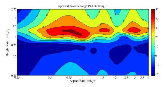
Figure 4.3. Change in power (caused by coupling) vs. aspect and height ratio caused by Kanai-Tajimi.
