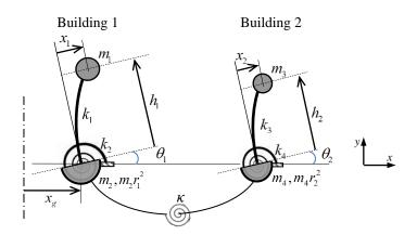
Figure 2.1. Two buildings discrete model
