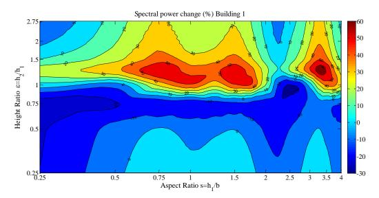
Figure 4.4. Change in power (caused by coupling) vs. aspect and height ratio caused by Westmorland.
