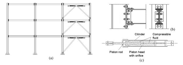
Figure 1.1. (a) Viscously damped steel frames. (b) Semi-rigid joints with angles. (c) Viscous fluid device
