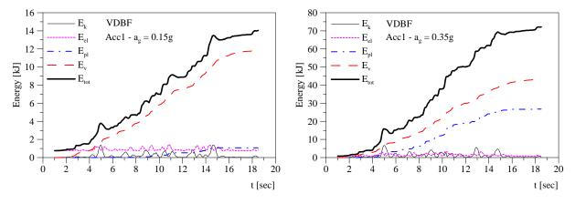
Figure 4.6. Time history of Energy for VDBF under Acc1 with  $a_g = 0.15g$  and  $a_g = 0.35g$  for frame with nonlinear viscous dampers
