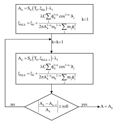
Figure 3.2. Iterative procedure to calculate displacement demand
