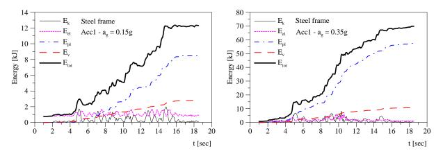
Figure 4.5. Time history of Energy for steel frame under Acc1 with  $a_g = 0.15g$  and  $a_g = 0.35g$  for steel frame
