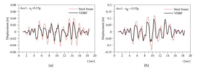
Figure 4.2. Time history of displacement at top floor for Acc1 with  $a_g = 0.15g$  and  $a_g = 0.35g$  for steel frame (a) and frame with nonlinear viscous dampers (b)
