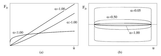
Figure 2.1. Force-velocity curves (a) and force-displacement curves (b) for viscous dissipation systems
