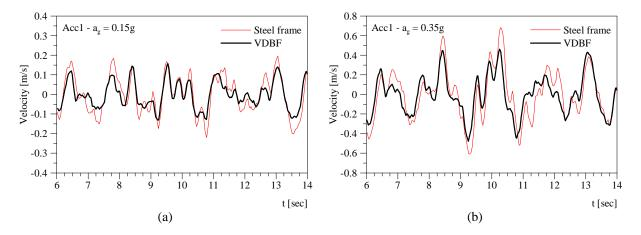
Figure 4.3. Time history of velocity at top floor for Acc1 with  $a_g = 0.15g$  and  $a_g = 0.35g$  for steel frame (a) and frame with nonlinear viscous dampers (b)
