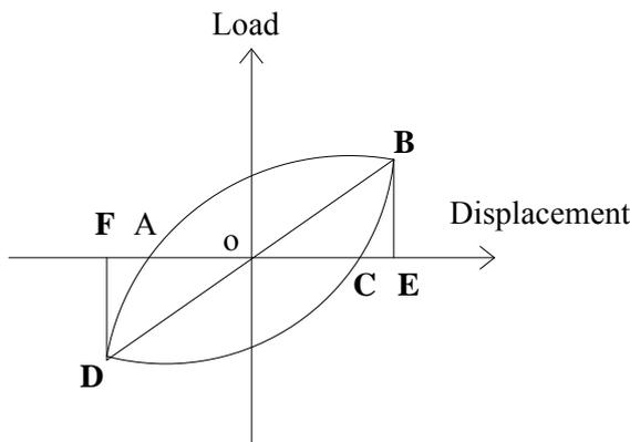
**Figure3.6** Load-displacement hysteretic loop
