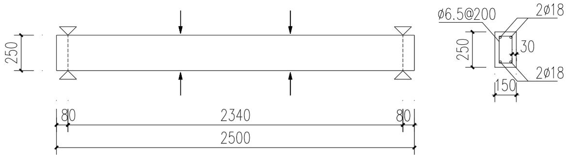
Figure 3.1 Dimension of the beam (unit: mm)
