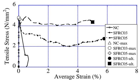
Figure 3. Splitting tensile strength – strain
