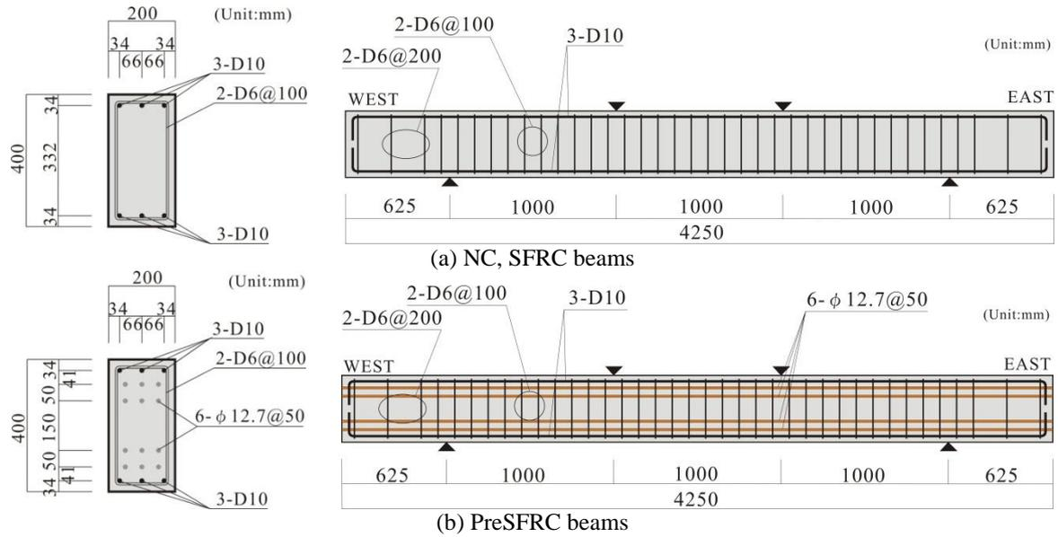
Figure 1. Details of specimen
