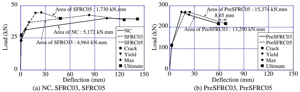
Figure 7. Comparison of toughness
