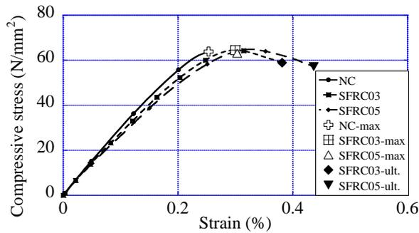
Figure 2. Compressive strength – strain
