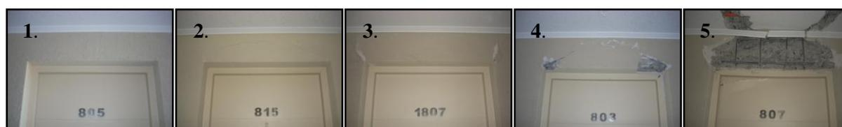
**Figure 5.** Damage states defined. 1. No observable damage. 2. At least one concrete crack. 3. Some cover concrete spalling. 4. Major cover concrete spalling. 5. Complete cover concrete spalling.
