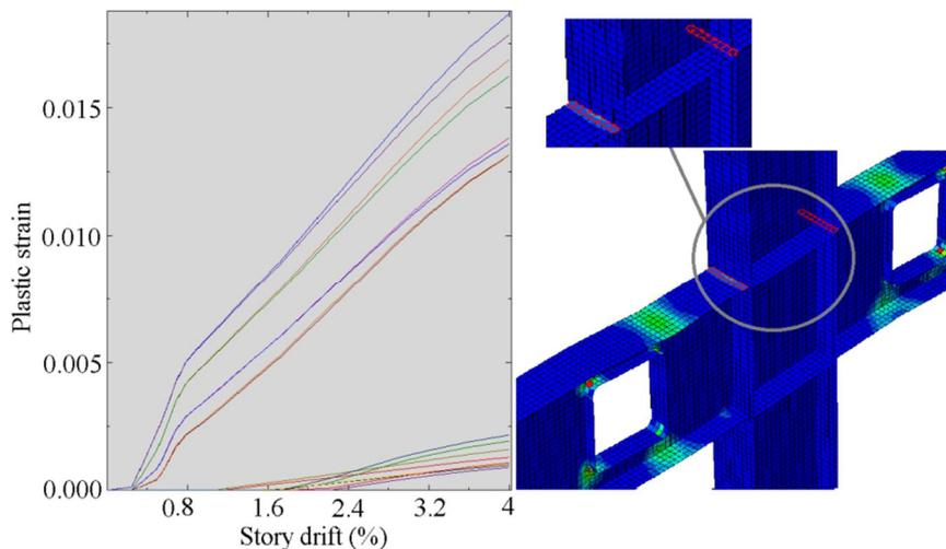
**Figure 3.1.** Progress of Plastic Strain of Selected Points vs. Story Drift
