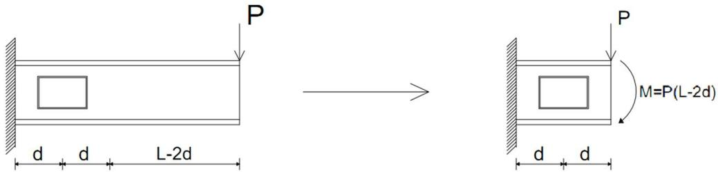
**Figure 4.2.** Effect of Span Length in the Magnitude of Moment Force
