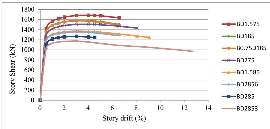
**Figure 3.2.** Diagram of Shear Force vs. Corresponding Displacement of Point A for Acceptable Models
