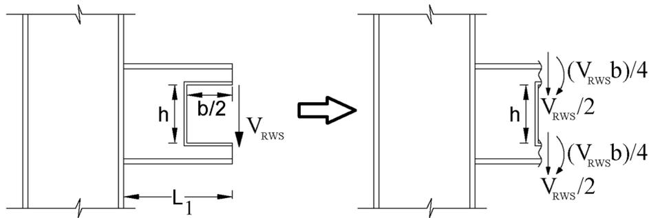
**Figure 5.1.** Pure Shear at the Center of Reduced Section
