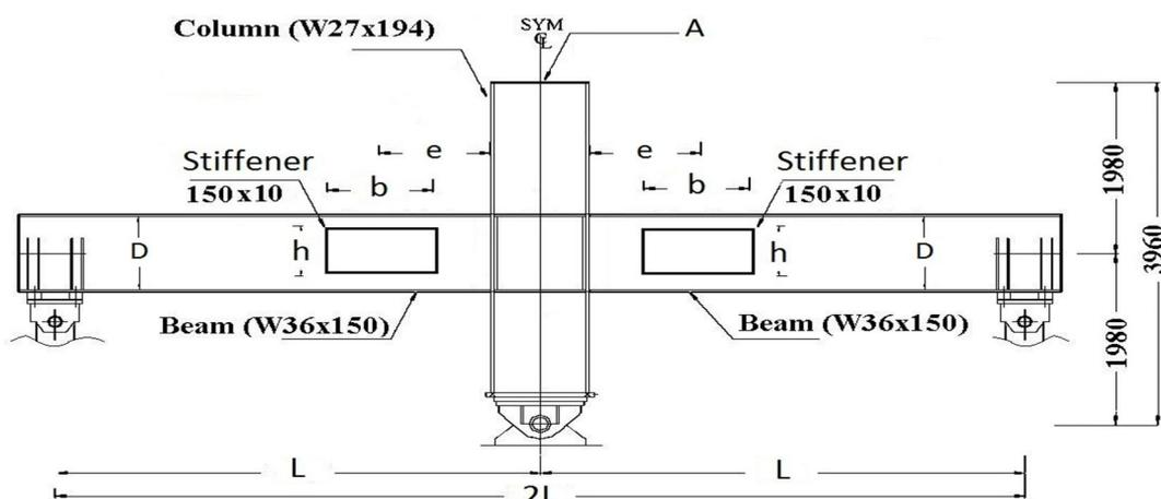
Figure 2.1. The Modeled RWS Connection (Dimensions in mm)
