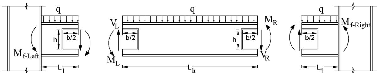
**Figure 5.2.** Structural Layout of Expected Forces of Beam
