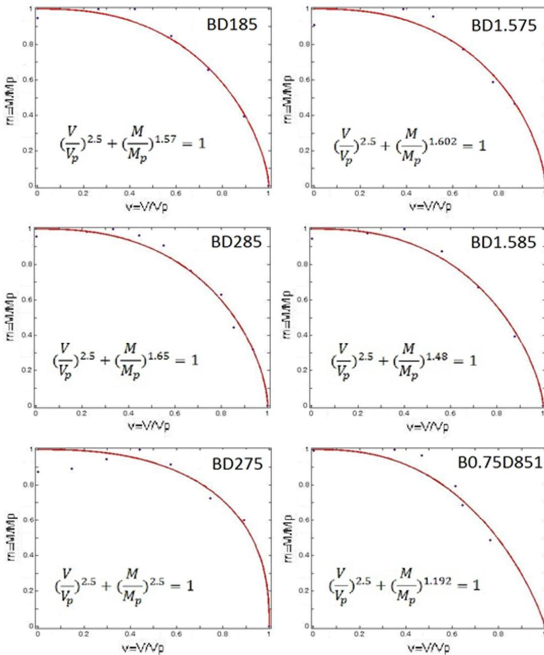
**Figure 4.1.** Interaction Curves and Equations for Each Model
