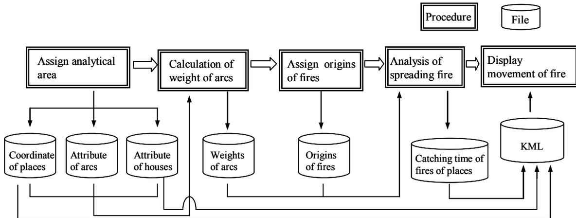
Figure 8. Procedure and related files in simulation system of earthquake-induced urban spreading fire
