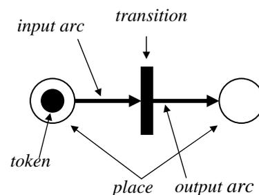
Figure 2. Base elements of Petri-net
