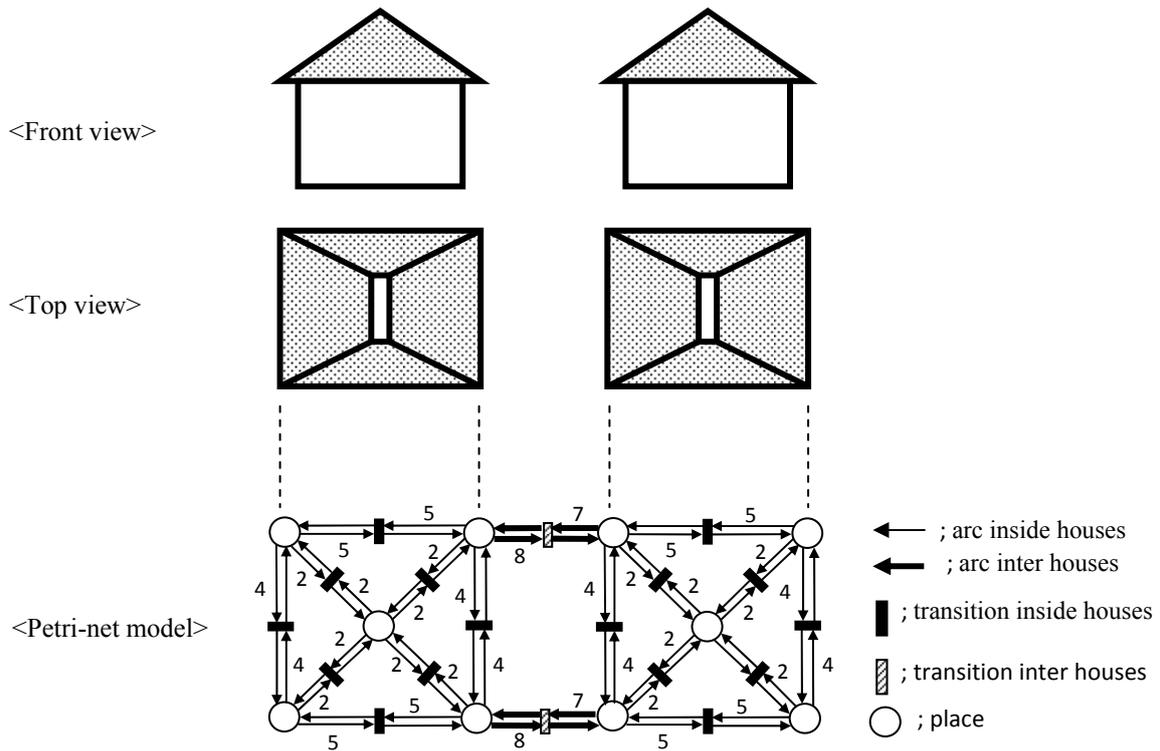
Figure 3 Petri-net modeling for simulation of spreading fire
