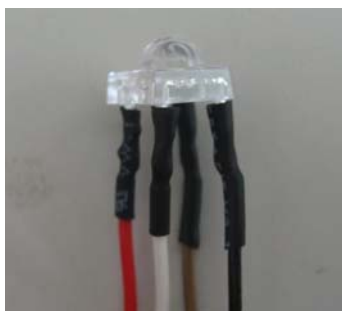
Figure 4. LED connectd by cable and sleeve
