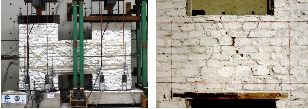
Figure 6.4. View of the second specimen at C19_38 ( \theta_n = 3\% ) on the left and close view of the crack pattern of the spandrel at the end of the test S2 on the right.
