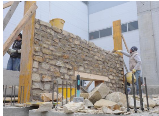
Figure 3.1. Dimensions of the two double-leaf stone masonry specimen [mm] (left) and picture taken during the construction on the first specimen (right)
