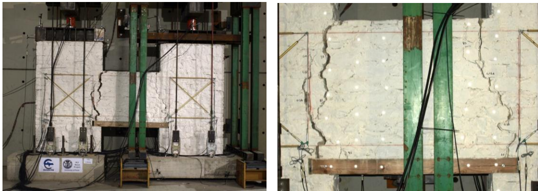
Figure 6.1. View of the entire specimen at C15 ( \theta_n = 1.5\% ) (left) and crack pattern of spandrel at C10 ( \theta_n = 0.6\% ) (right)
