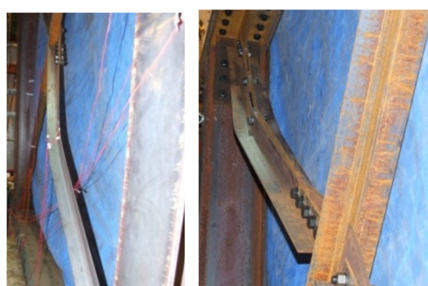
Figs.3.3 Buckling at the story drift of 0.005 rad.
