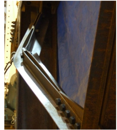
Fig.3.5 Break point of 2L-75x6 brace
