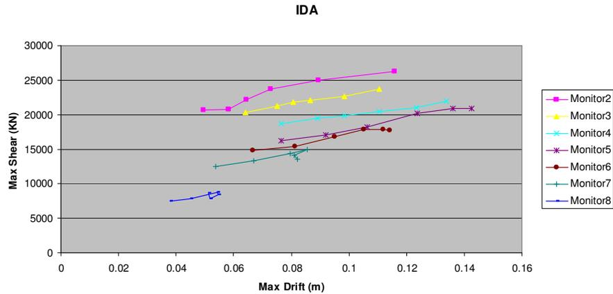
**Figure 5.** The total shear from columns of the same storey function of the interstorey drift between nodes at the top and at the bottom of the same storey (of the middle column of the middle frame; i.e. internal frame) drawn for all stories.
