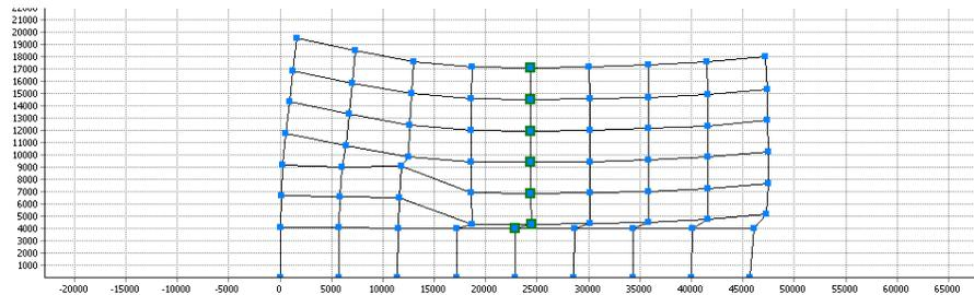
**Figure 4.** The deformation for a scaling factor of 92.745 under adaptive pushover analysis.
