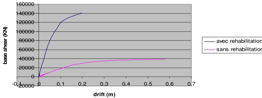
**Figure 8.** Displacement between the roof and the base nodes in the East – West direction function of the base shear.
