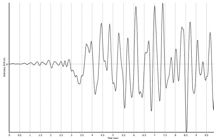
**Figure 7.** Displacement between the roof and the base nodes in the EAST – WEST direction function of the time.
