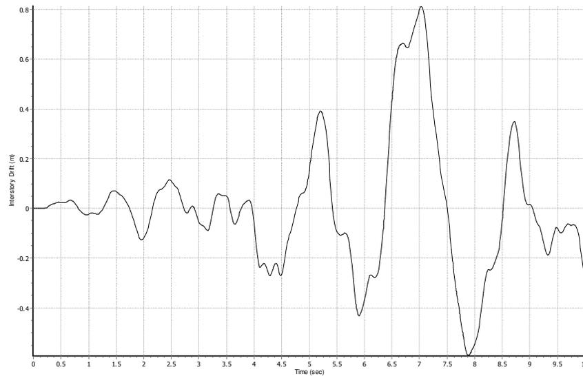
**Figure 3.** Lateral displacement, or drift, between the roof and base node of central column of internal frame of the East – West façade in the direction x with respect to the time, for San Fernando Earthquake.
