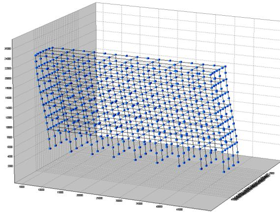
**Figure 1.** The structure model in 3D deformed for the time of 7.344 seconds, under Northridge time history record
