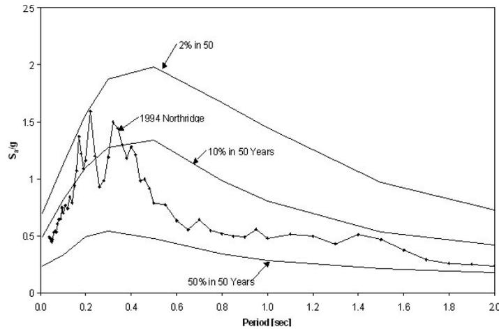
**Figure 6.** Site-specific response spectra for seismic hazards with a probability of exceedance of 2%, 10%, and 50% in 50 years, along with the 1994 Northridge Earthquake data, PEER 2005/11.
