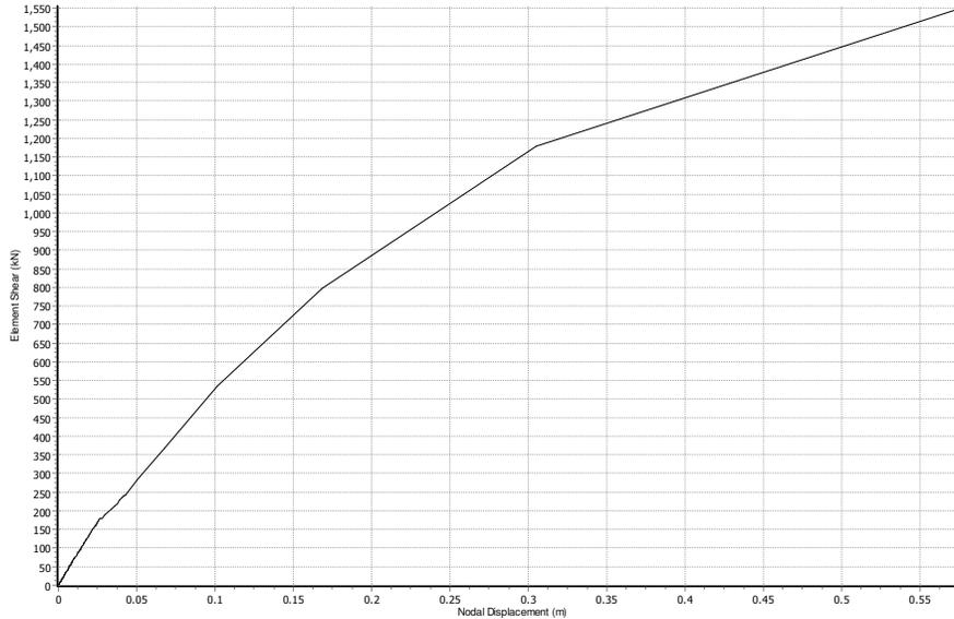
**Figure 2.** The roof lateral displacement of central column of internal frame of the East – West façade in the direction x, with respect to the element base shear.
