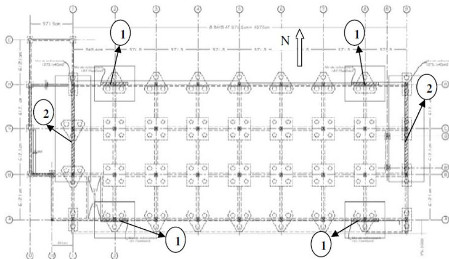
**Figure 9.** Plan of the foundation after retrofitting; number 1 indicates the walls of 12.75m x 0.4m on the East – West direction and number 2 indicates the walls of 3.52m by 0.4m on the North – South direction.
