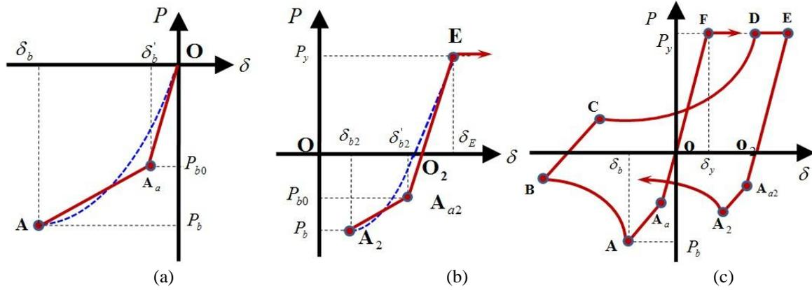
**Figure 1.** Relationship between axial force and displacement of a brace under cyclic load: (a) Local modified phases (OA); (b) local modified phases (EA<sub>2</sub>) and (c) modified hysteretic curve.
