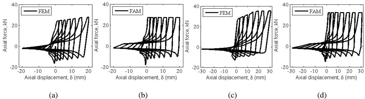
**Figure 4.** Hysteretic curves of two braces under axial force using: (a) set 1 with FEM; (b) set 1 with FAM; (c) set 2 with FEM; (d) set 2 with FAM
