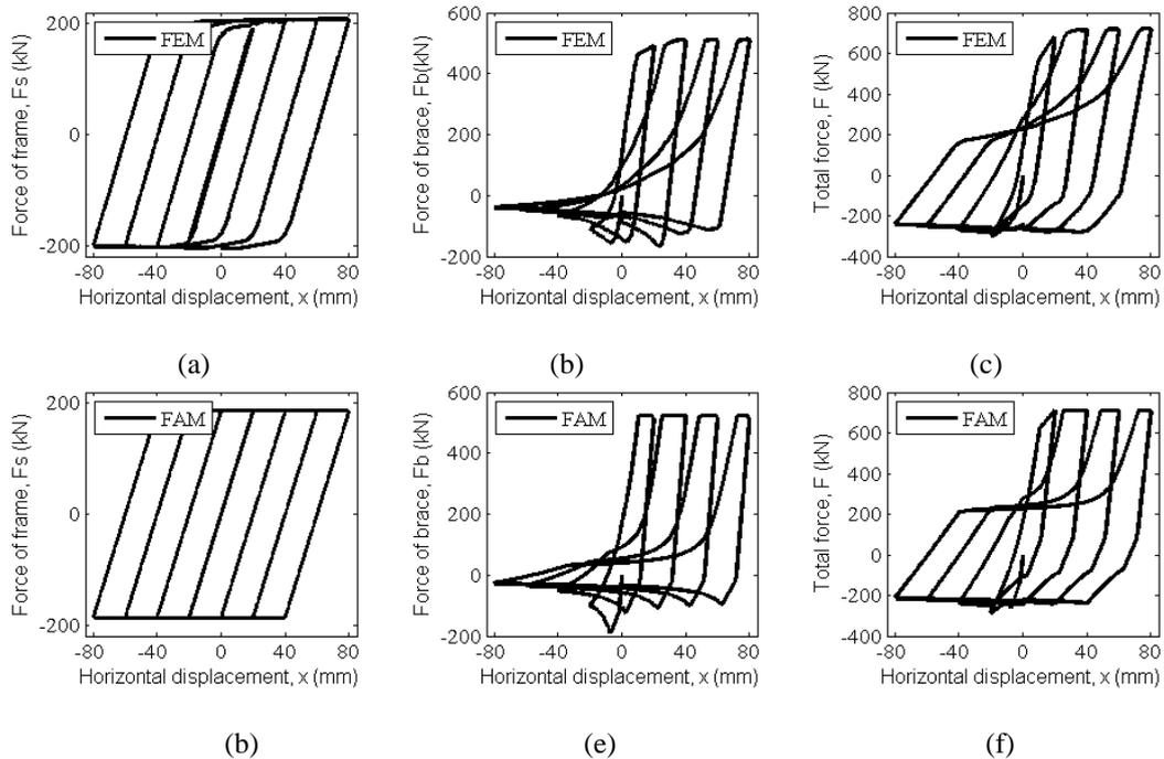
**Figure 6.** Comparison of the hysteretic behavior of the frame, brace and CBF using FAM and FEM: (a) frame (FEM); (a) brace (FEM); (a) CBF (FEM); (a) frame (FAM); (a) brace (FAM); (a) CBF (FAM).
