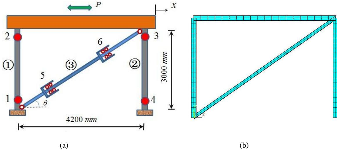
**Figure 5.** An example of one-storey CBF: (a) FAM model and (b) FEM model
