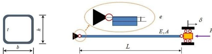
**Figure 3.** Geometric parameters of brace
