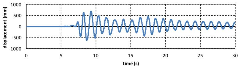
**Figure9.** Displacement time history of the tower top (seismic response analysis)
