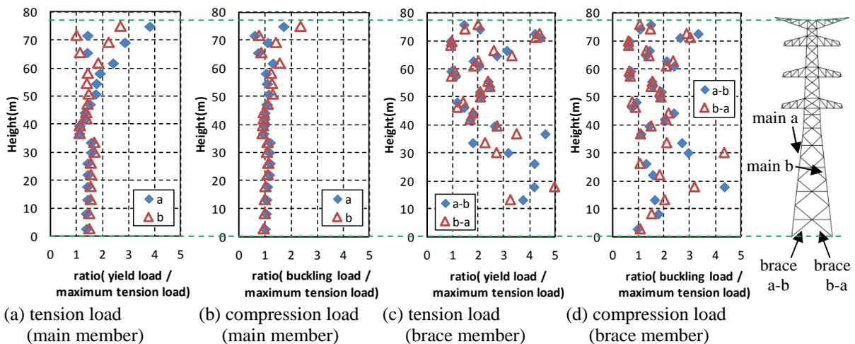
**Figure12.** Maximum tension and compression axial forces for each panel (seismic response analysis)
