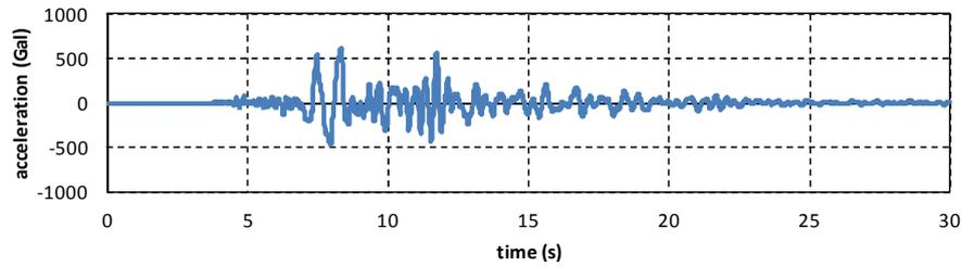
**Figure3.** Ground motion record (JMA Kobe, EW component)
