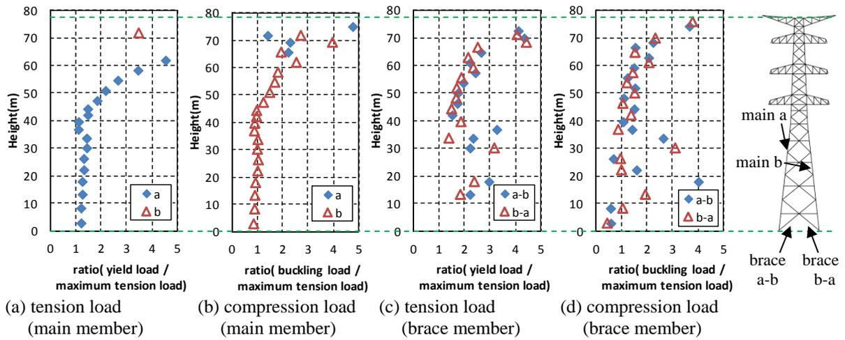
**Figure8.** Maximum tension and compression axial forces for each panel (wind response analysis)
