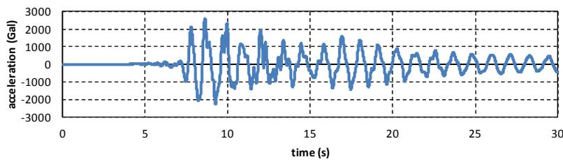
**Figure10.** Acceleration time history of the tower top (seismic response analysis)
