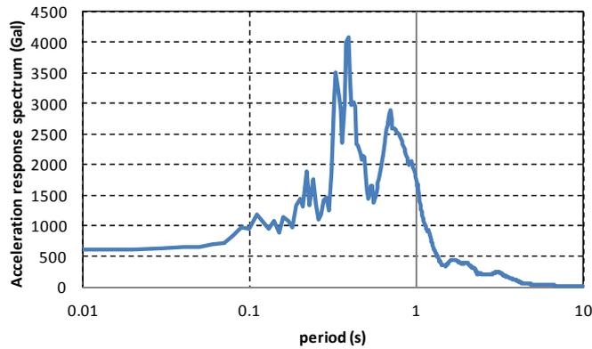
**Figure4.** Acceleration response spectrum of JMA Kobe (h=0.01)
