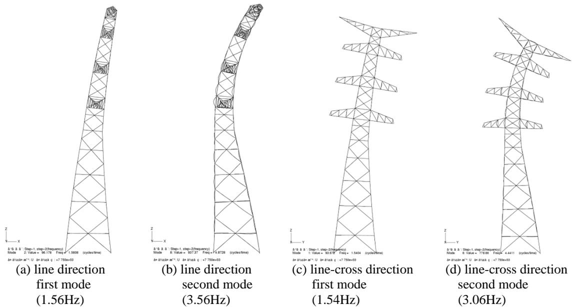
**Figure 6.** Mode shapes and natural frequencies of the target tower
