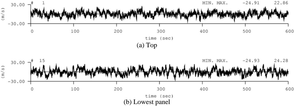
**Figure5.** Fluctuating wind velocity of the tower top and lowest panel
