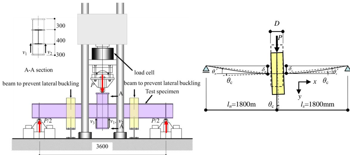
Figure 2.3 Loading apparatus and the method of measurement
