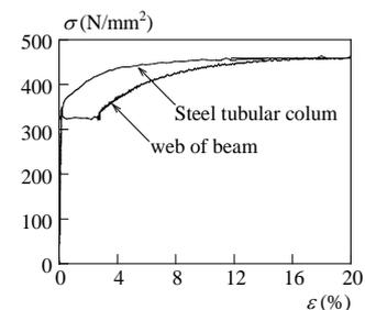
(a) Steel tubular column and beam web
