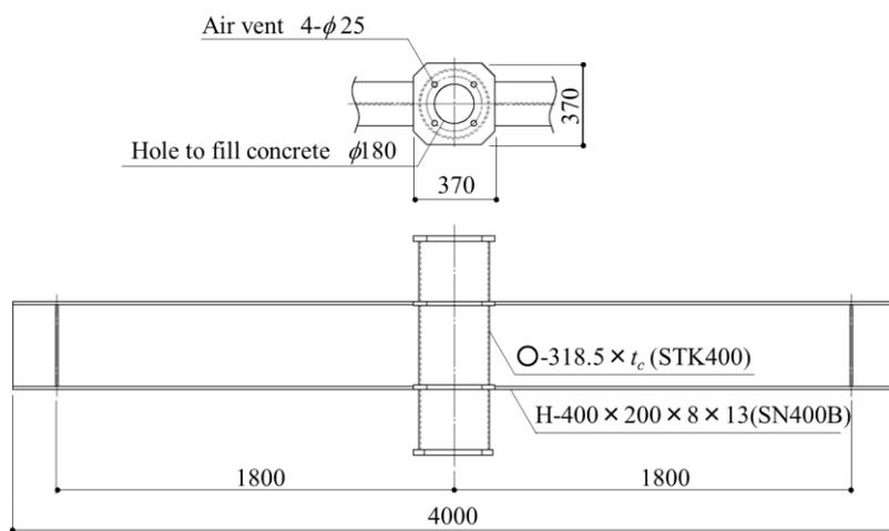
Figure 2.1 The shape of the specimen
