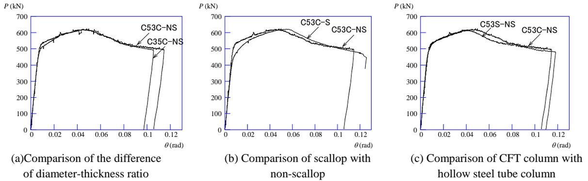
**Figure 3.1 Load  $P$ -slope angle  $\theta$**
