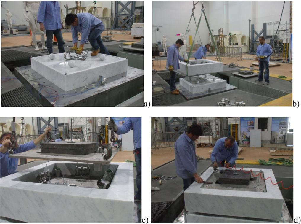
**Figure 4.** a) lower block and recentering device, b) upper block with vertical isolation
