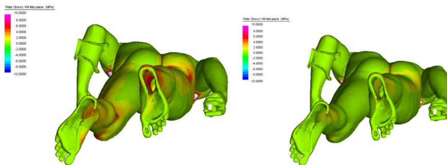
**Figure 15.** Bronze A: comparison of the stress fields by the old and new strengthening forces
