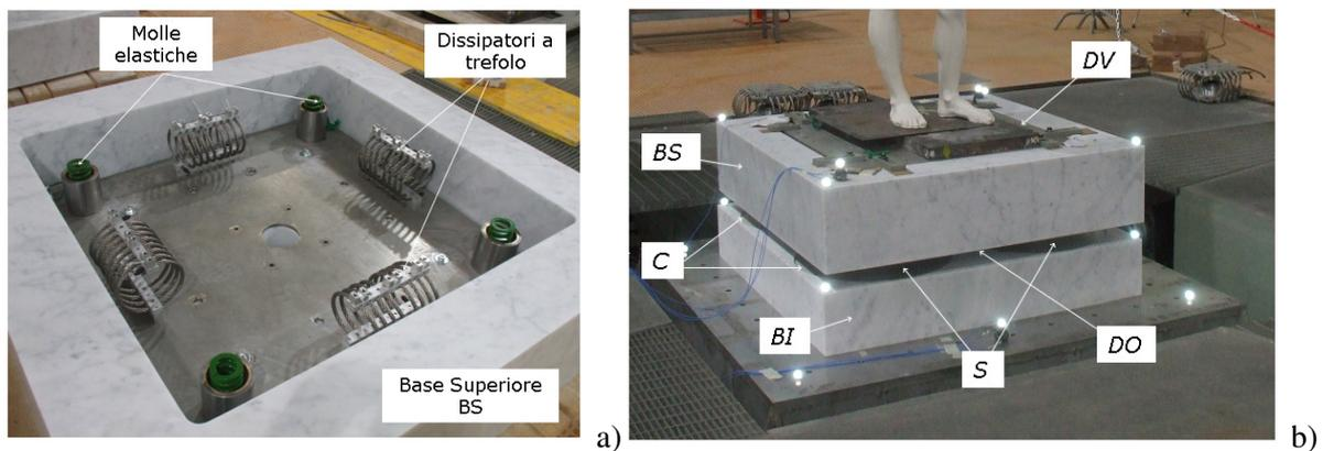
**Figure 3.** marble basement for the bronzes of Riace: a) details of the vertical isolation device inserted into the upper block, b) basement ready for the shaking table tests
