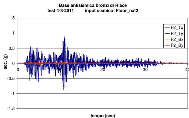
**Figure 8.** shaking table test Floor-Nat2: F2\_Tx,y= base table, F2\_Bx,y= basement. Isolation Coeff.= 20.
