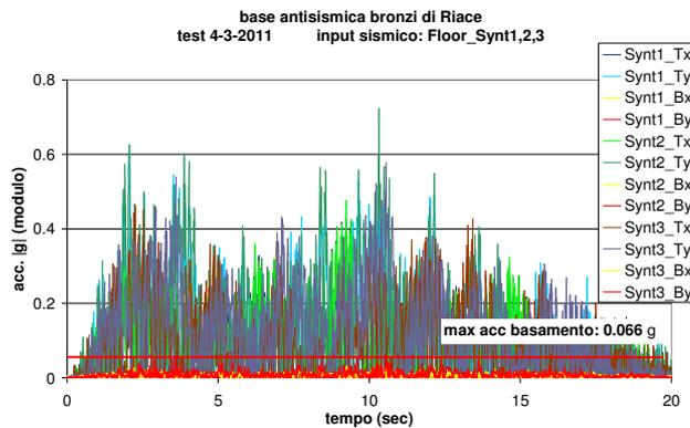
**Figure 10.** shaking table test Floor\_Synt1, Floor\_synt2 and Floor\_synt3: T= base table, B= basement
