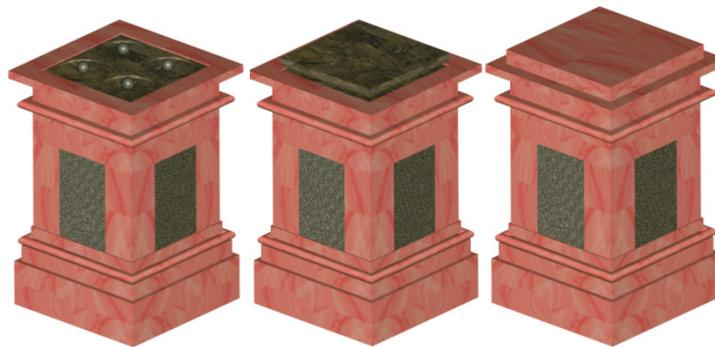
**Figure 18.** The granite anti seismic basement for the “Annunciazione” by Francesco Mochi. The granite is covered by the same marble of the original basement
