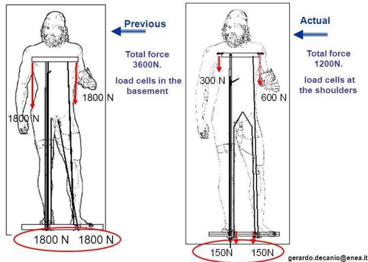
**Figure 13.** The previous rubber bearing devices required the application of strengthening forces
