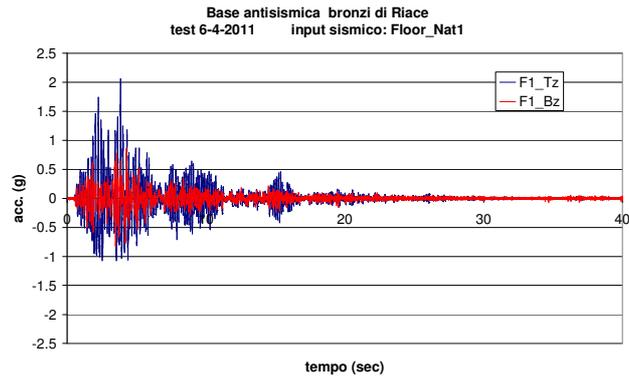
**Figure 9.** shaking table test Floor-Nat1: F1\_Tz= base table, F1\_Bz= basement. Isolation Coeff.= 2.4
