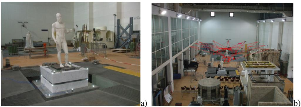
**Figure 5.** Shaking table tests of the marble anti seismic basements for the Bronzes of Riace
