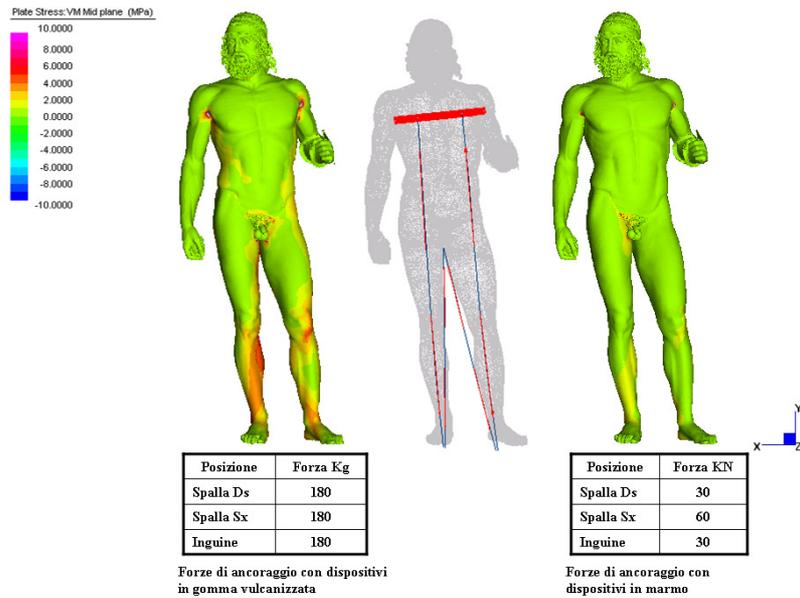
**Figure 14.** Bronze A: comparison of the stress fields induced by the new and old strengthening forces
