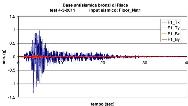
**Figure 7.** shaking table test Floor-Nat1: F1\_Tx,y= base table, F1\_Bx,y= basement. Isolation Coeff.= 22.
