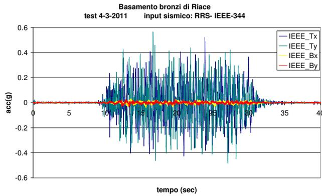
**Figure 11.** shaking table test IEEE-344: T= base table, B= basement
