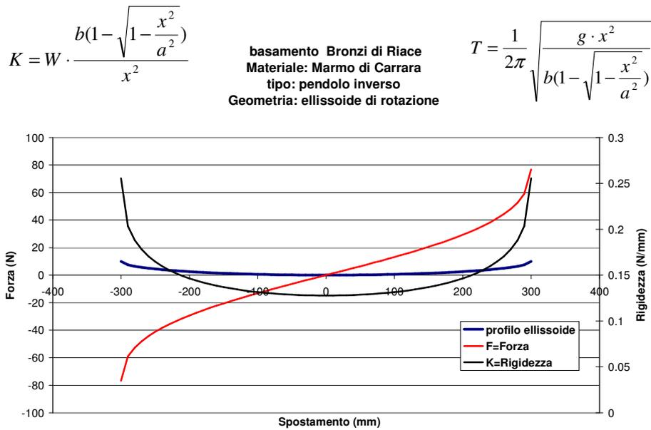
**Figure 2.** design parameters for the sliding surfaces: K=stiffness, W=weight, T=period
