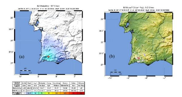
Figure 3.1. Shakemaps for 12 km NNE of Silves earthquake  $(37,29^{\circ}N; 8,42^{\circ}W)$ , on 2011-03-26, ML = 4,0: (a) Instrumental Intensity; (b) PGA. The epicentre is shown with a red star. The triangles shown the seismic stations.
