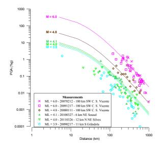
Figure 2.2. Attenuation relations expressed as PGA (for Imm < V), determined using the relation proposed by Miranda (personal communication). The symbols represent the values of PGA (%g) observed for each earthquake listed in the legend at bottom left.
