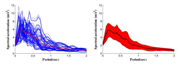
**Figure 2.7.** Left: acceleration response spectra computed for each of the 100 simulations and mean spectrum (thick red line). Right: mean and mean plus/minus one standard deviation (area) acceleration response spectra.
