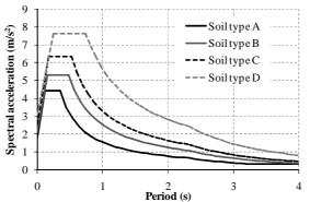
Figure 2.2 Response spectra for different soil conditions according to NTC08 for Teramo (Central Italy).
