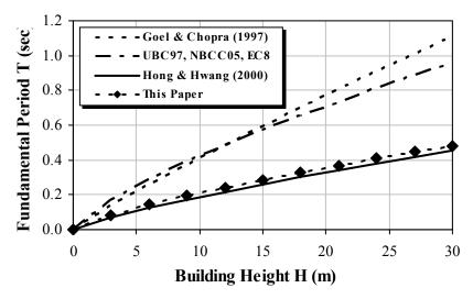
**Figure 8.** Comparison between Code, Goel & Chopra (1997), Hong and Hwang (2000) formulations with the regression obtained from the analysis of Canadian data (this paper).
