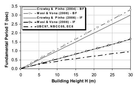
**Figure 1** Estimation of fundamental period of RC buildings having frames with (IF, Infilled Frame) and without (BF, Bare Frame) infills walls. Comparison with Code (UBC97, NBCC05, EC8) previsions.
