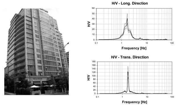
**Figure 4**. On the left: Marriott Hotel in Victoria. On the right: HVSR curves for the ambient vibration signals recorded on the longitudinal (Long) and transversal (Trans) direction of monitored building as a function of the vibration frequency. The mean value of H/V has been reported with  $\pm 1\sigma$  (standard deviation).
