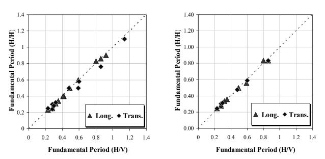
**Figure 6.** On the left: comparison between the fundamental periods estimated from HVSR and HHSR (measure on the basement) techniques for the two orthogonal directions (see text for details). On the right: comparison between the fundamental periods estimated from HVSR and HHSR (measure on free-field) techniques for the two orthogonal directions (see text for details).
