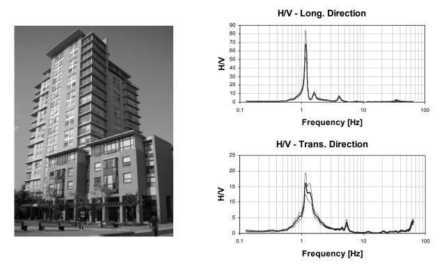
**Figure 5**. On the left: Student House in Vancouver. On the right: HVSR curves for the ambient vibration signals recorded on the longitudinal (Long) and transversal (Trans) direction of monitored building as a function of the vibration frequency. The mean value of H/V has been reported with  $\pm 1\sigma$  (standard deviation).
