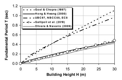
**Figure 3.** Comparison between Code, Goel & Chopra (1997) and the results of empirical studies based on ambient vibration measurements.
