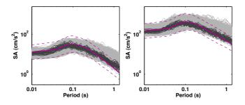
**Figure 4.2.** Comparison of simulated (gray lines) and predicted (purple line) acceleration response spectra corresponding to (left) M<sub>W</sub>=5, R<sub>RUP</sub>=50km and V<sub>S30</sub>=550m/s; and (right) M<sub>W</sub>=6.6, R<sub>RUP</sub>=30km and V<sub>S30</sub>=550m/s. In light gray lines, the 2500 simulations and in dark gray lines, the 30 best matched time-histories.
