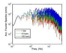
Figure 4.1. Simulated acceleration Fourier spectra for different values of stress drop.
