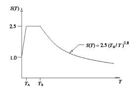
Figure 3.1 Spectrum Function
