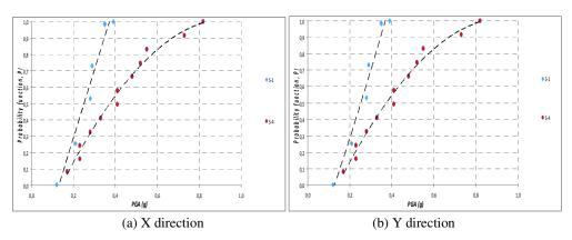
Figure 4.2 Development of fragility curves for Building 2 in both X and Y directions
