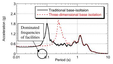
Fig.1 Floor response spectrum of two isolation systems
