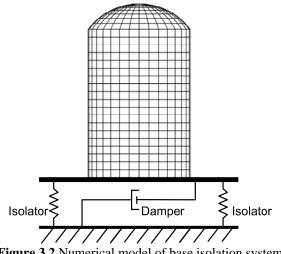
Figure 3.2 Numerical model of base isolation system
