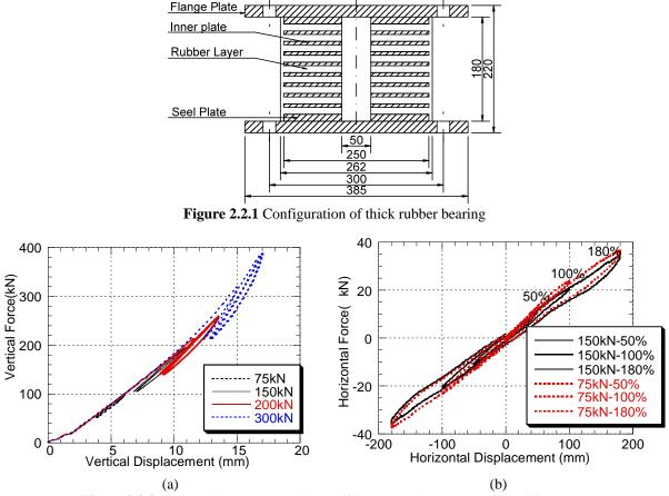
Figure 2.2.2. Hysteretic curves: (a) Shear stiffness test; (b) Compressive stiffness test
