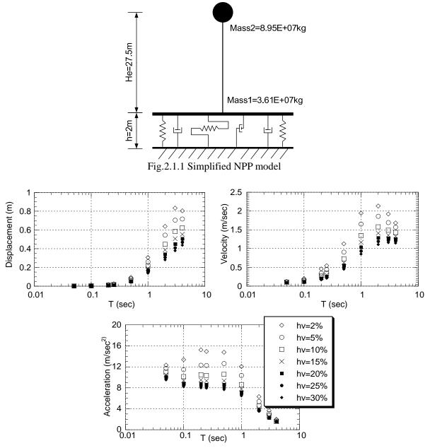
Fig.2.1.2 Seismic responses of simplified NPP model
