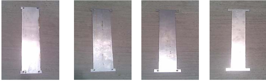
Figure 5. Columns used to simulate damage (10, 20, 30 and 40% area reduction)
