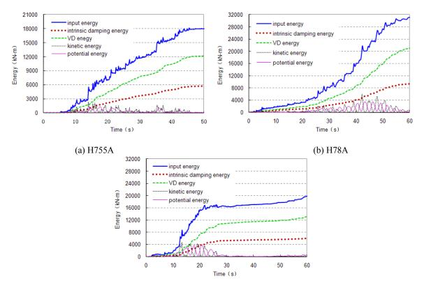
(c) H78B Figure 4.5 Energy dissipation categories under minor earthquake
