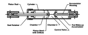
Figure 2.1 Viscous Damper Sketches
