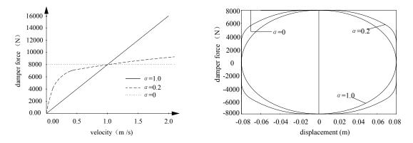
Figure 2.2 Relationship of damper force and velocity
