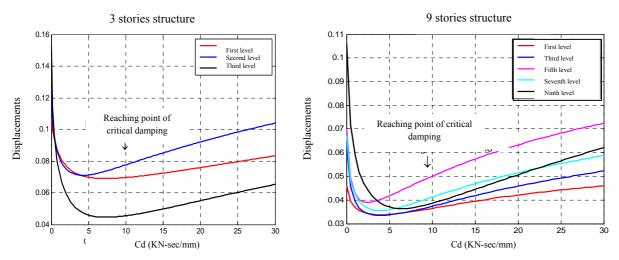
Figure 9. Variation of the displacements for 3 and 9 SAC structures.
