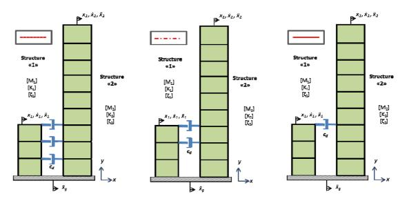
Figure 12. Models used to determine optimal position of the damper.
