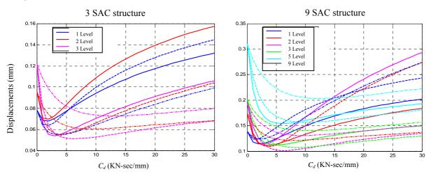
Figure 11. RMS displacement responses for the different positions of the dampers.
