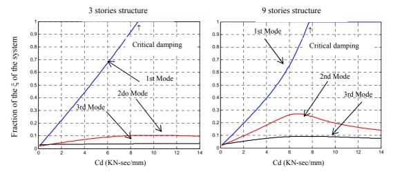
Figure 8. Variation of the critical damping of the system.
