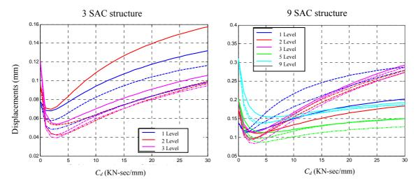
**Figure 13.** RMS displacement responses for the different number of the dampers.
