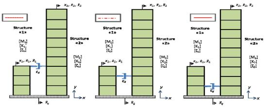
Figure 10. Models used to determine the best position of the damper.
