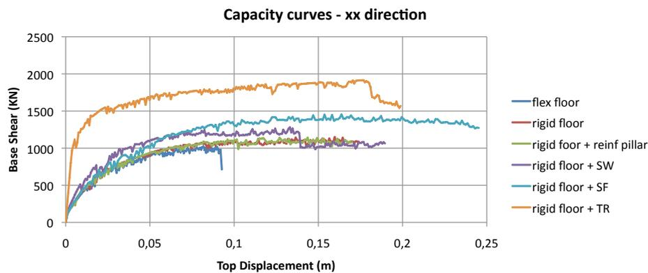
Figure 5.1. Pushover curves comparison in the xx direction
