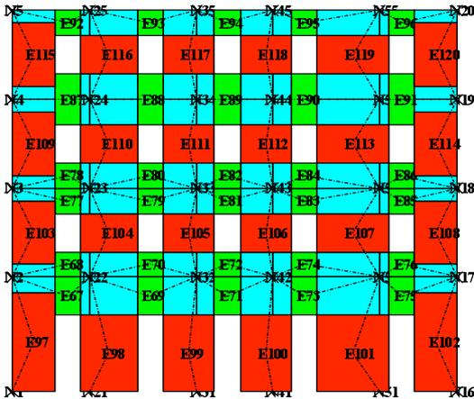
Figure 2.3. Equivalent frame idealization of back façade (P4)
