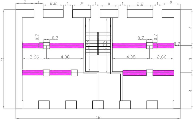
Figure 3.2. Positioning of the eight steel frames on the ground floor – units in metres
