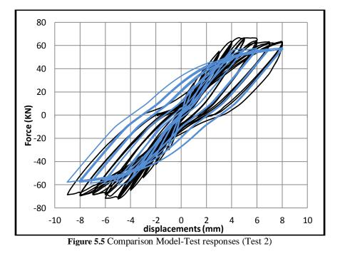
The global behavior is well reproduced as shown in Fig. 5.5. After the plastification of the longitudinal reinforcements, the form of cycles evolves according to steel behavior.
