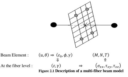
The hypothesis of plane sections (Timoshenko theory) allows expressing the displacements u(x, y, z), v(x, y, z), w(x, y, z) of any node of the beam as a function of the "sections variables"
