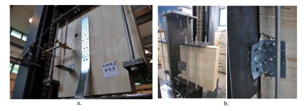
Figure 3.1. Experimental setup of hold-down loaded in tension (left a.); angle bracket loaded in shear (right b.)
