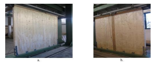
Figure 3.2. Experimental setup of full-scale X-Lam wall panels subjected to horizontal load - single wall (left, a.) and coupled wall with LVL spline vertical joint (right, b.)
