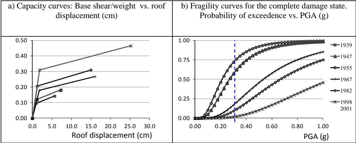
**Figure 3.** Capacity and fragility curves for a standard two-story reinforced concrete school building located in Caracas on stiff soil, for each building code since 1939 to 2001.
