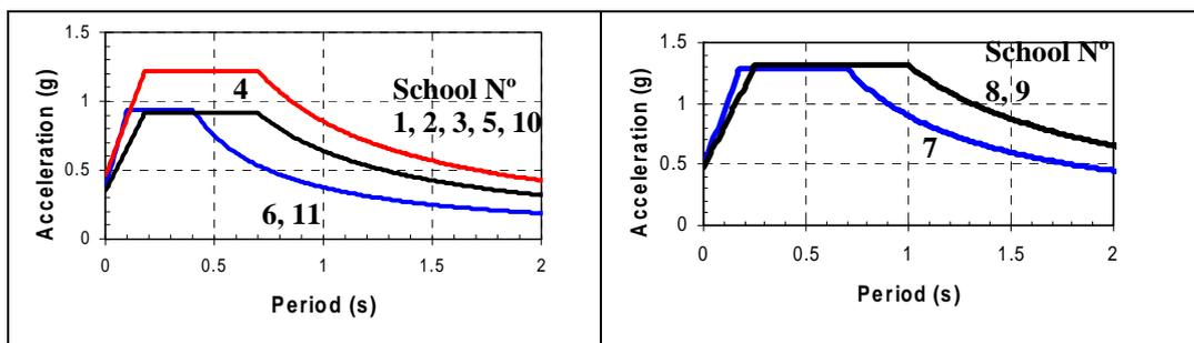
**Figure 7.** Elastic response spectra for evaluation and retrofitting at each school.
