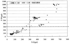
Figure 5. Relationship Diagram between Seismic Acceleration and Damage Degree of Adobe Masonry. (Chang, J. S. et al., 2001)
