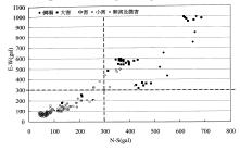
Figure 4. Relationship Diagram between Seismic Acceleration and Damage Degree of Brick Masonry. (Chang, J. S. et al., 2001)
