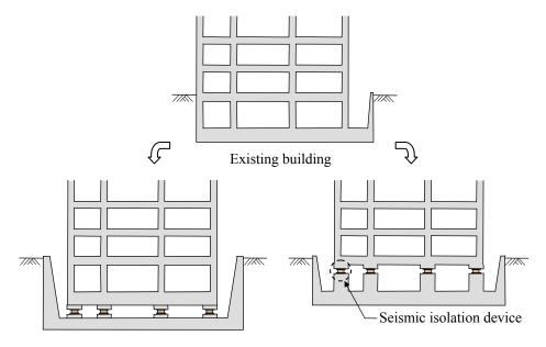
a) A case to install under the foundation b).
