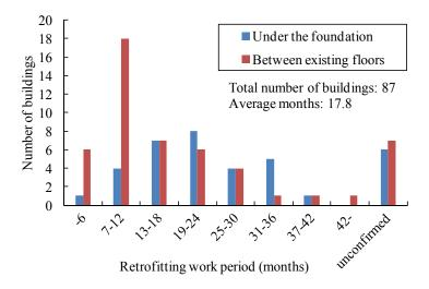
Figure 2.3.4. Distribution of the periods for the seismic isolation retrofitting work
