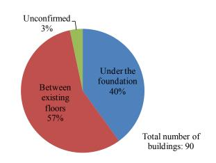
Figure 2.3.2. Ratio of the location of seismic isolation layer
