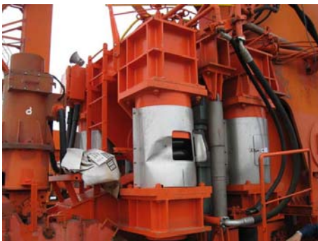
Figure 24. Damage due to collisions with floating objects (Provided by JCA)
