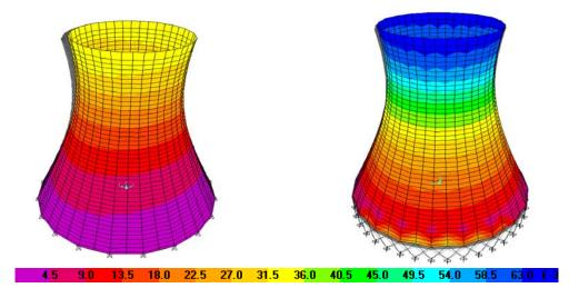
Figure 6. 3D Modeling of Radial displacements along the height of the tower for FBA, CSA
