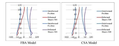
Figure 5. Radial displacements along the height of the tower for FBA, CSA
