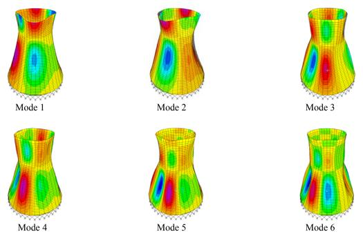
Figure 4. Variation of Deformed Shape CSA Mode 1,2,3,4,5,6
