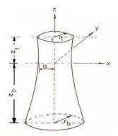
Figure 1. Cooling tower geometry (After Fonder and Clough, 1973)
