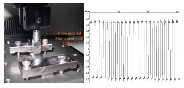
Photo 2. Experimental test setup
