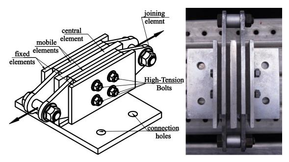
Figure 1. Basic layout of the device
