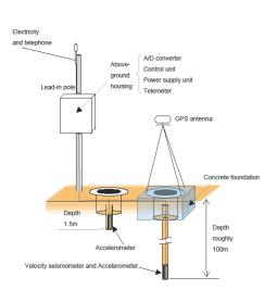
Figure 2. Configuration of the AN-net station
