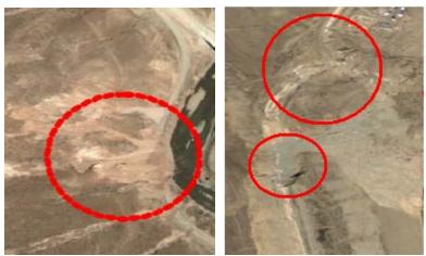
Figure 2.Interrupted road by landslide and collapsing
