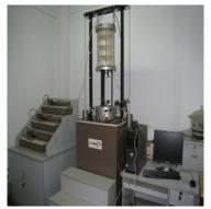
(a) Hollow cylinder apparatus
