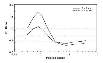
Figure 4.1. Vertical-to-horizontal spectral ratio (after Bozorgnia and Campbell, 2004a).
