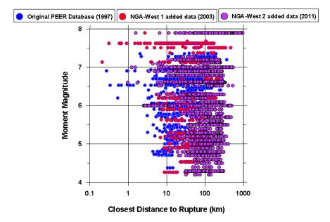
Figure 2.1. Magnitude-distance representation of the PEER ground motion databases since 1997.
