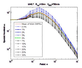
**Figure 5.1.** The geometric mean of the five NGA GMPEs (red) is scaled to adjust for various damping ratios from 0.5 to 30%. Assumptions: reverse fault, dip = 45°, hanging wall, fault rupture width = 15km,  $R_{jb}$ =0km,  $R_x$ =7km (after Rezaeian et al, 2012).
