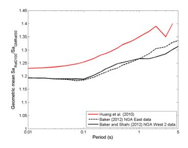
Figure 7.1: Geometric mean ratios of  $Sa_{RotD100}/Sa_{GMRott50}$  in stable continental regions from Huang et al. (2010) and the NGA East project (Baker 2012), compared with the equivalent Shahi and Baker (2012) ratios for active shallow crustal tectonic regions (after Baker, et al., 2012).
