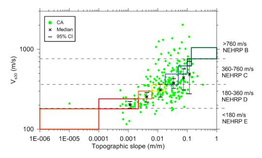
**Figure 6.**  $V_{s30}$  versus slope from California data and estimates from Wald and Allen (2007) for active tectonic regions. Color coded polygons correspond to slope ranges within NEHRP classes.
