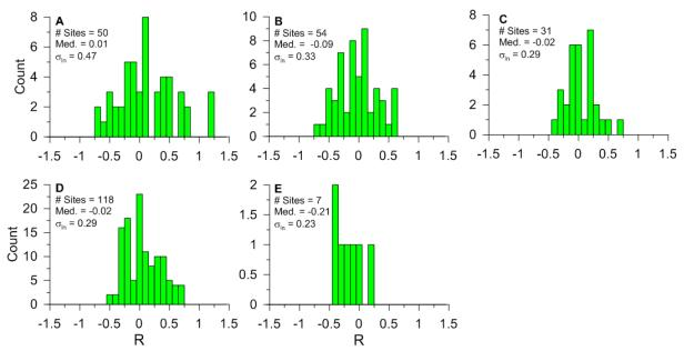
**Figure 5.** Residuals of  $V_{s30}$  from estimates based on the geotechnical proxy (Geomatrix third letter) using the methods of Chiou et al. (2008). Based on  $V_{s30}$  measurements and  $V_{sz}$ - $V_{s30}$  relations.
