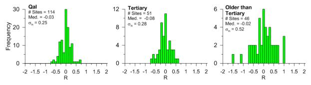
**Figure 4.** Residuals of  $V_{s30}$  from estimates based on the geology proxy using the methods of Wills and Gutierrez (2008) for alluvium and Wills and Clahan (2006) for all other conditions.
