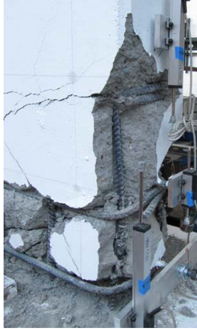
Figure 7. Local Buckling of Vertical Bars and Opening of Hooks
