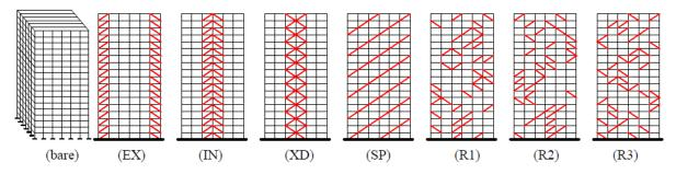
Figure 2. Tested Bracing Arrangements of the Perimeter Concrete Frame (Mezzi 2010)
