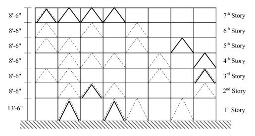
Figure 4: Van Nuys Hotel schematic with Sequential Search (Solid Lines) and Genetic Algorithm (Dashed Lines) optimized retrofit schemes
