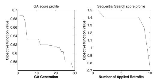
Figure 3: (a) Genetic Algorithm and (b) Sequential Search improvement at each iteration, note the separate vertical axes
