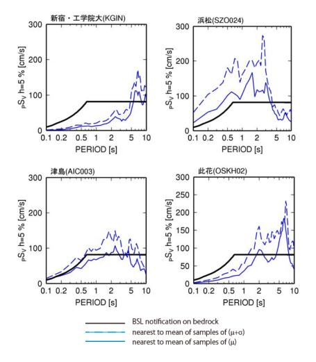
Figure 6. Pseudo velocity response spectra for simulated motions for three-connected earthquake for 4 stations
