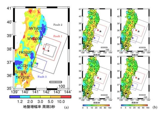
**Figure 6.** (a) The three macroscopic fault source models representing the 2011 Tohoku earthquake. The coloured contour shows the revised site amplification factor for Sa at 3 second of period. (b) left the pseudo velocity response spectra (pSv) at period 3 and 5 second with recorded motions for main shock, (b) right the pSv at 3 and 5 second for simulated motions with revised formula for main shock. (pSy are all with 5% damping)
