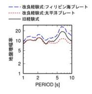
**Figure 3.** The difference of site amplification ratios of the K-NET site TKY018, in Tokyo. The black solid line is for the original formula Eqn. 2.1, the two dotted lines are for the revised formula Eqn.2.2. In addition, the blue dotted line is for events in the Philippine plate, whereas the red dotted line is for events in the Pacific plate.
