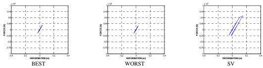
Figure 7. Hysteretic response of a representative bearing caused by the three input motion scenarios in the fiber element model of the bridge columns using OpenSees for the closed-gap analysis
