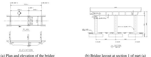
**Figure 1.** Configuration of the first (bridge no. 1) of the seven seismic design examples presented by the Federal Highway Administration (1996)
