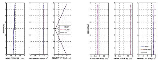
(a) Column absolute force demand envelopes in the lumped plastic hinge model using DRAIN-3DX
