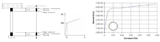
(a) Configuration of lumped plastic hinges
