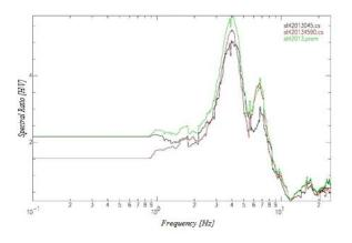
Figure 2. Spectral ratio[H/V], E-W direction, windows of 45 s. Reforma Avenue and 23 Sur Street
