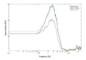
Figure 1. Spectral ratio [H/V], N-S windows of 45 s. 10 Poniente Street and 29 Norte Street
