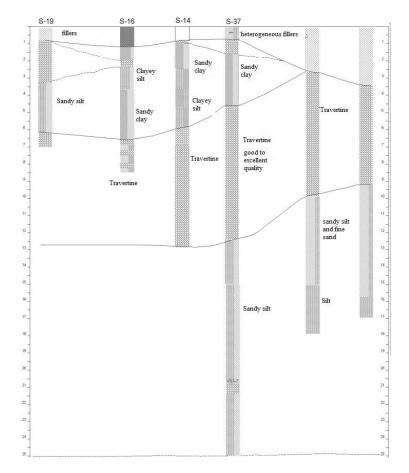
Figure 7. Stratigraphic layer 2. Reforma Avenue, between 7 and 4 Norte Street
