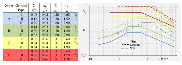
Figure 2. Spectrum designs according with CFE (1993).
