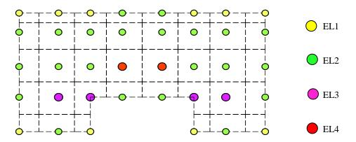
Figure 9. Isolated distribution and tributary areas to each four define types of isolated systems.
