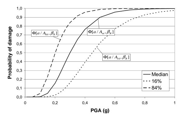
Figure 2. Example of lognormal fragility curves for a given damage level and for three different confidence levels
