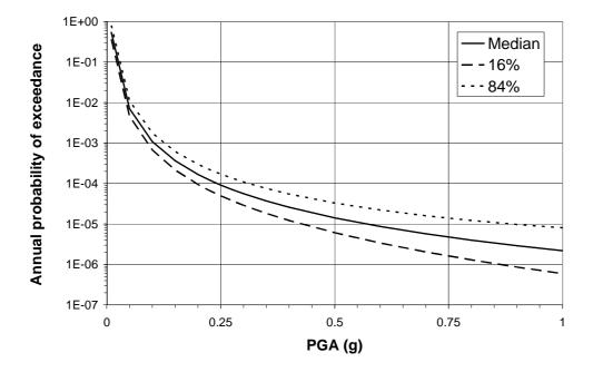
Figure 1. Example of seismic hazard curve in PGA
